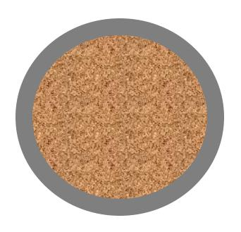
RAP aggregate with oxidized binder film
